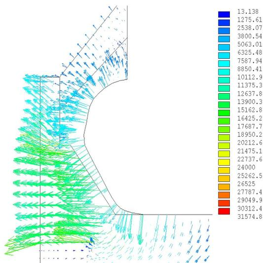
**Figure 4: Heat flux of side profiled carbon block**
